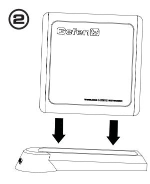
To place a main unit into a stand, first orient the front of the stand (where the logo is located) with the LED's on the front panel of the main unit. Lower the unit into the stand. There are channels (a) located on both the main unit and stand that will help guide the main unit into the stand.
