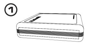
A vertical stand is included for placing the each main unit in an upright position. Vertical orientation is preferred because of the way that the radio waves are transmitted/received. Remove the main units and the stands from the packaging.
