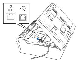
Carefully guide the network cable to the trench as shown below, following the trench around and toward the back of the machine. Then, connect the cable to your network.
