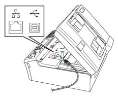
Carefully guide the USB cable into the trench as shown below, following the trench around and toward the back of the machine. Then, connect the cable to your Macintosh<sup>®</sup>.
