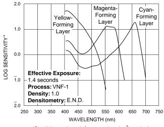
\*Sensitivity = reciprocal of exposure (ergs/cm<sup>2</sup>) required F002\_0150AC to produce specified density
