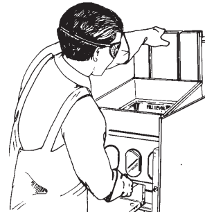
Fryer vessel being removed.
