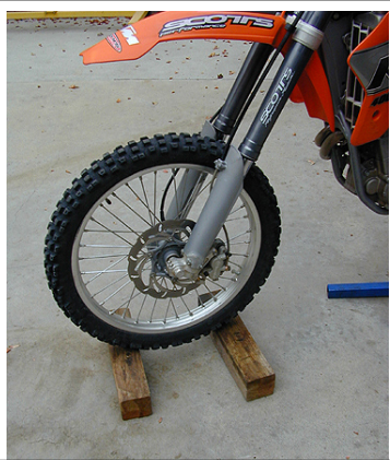
Block the front wheel & forks
