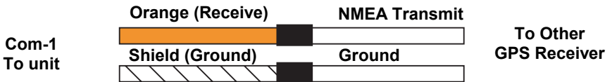
Com-1 wiring to receive NMEA position information from some other GPS receiver.
