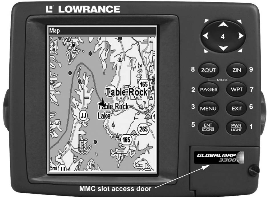
GlobalMap 3300C GPS unit, front view, showing full map, keyboard and access door for the MMC slot.
