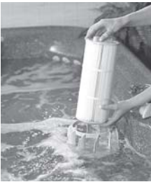
1) Center filter cartridge over canister
