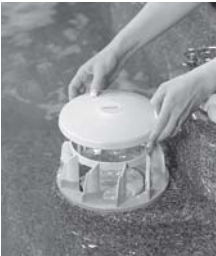
3) Snap Vortex filter top in place
