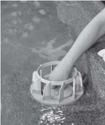
2) Screw filter cartridge in place
