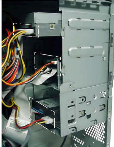
Fig. 5: Disconnecting power and data cables
