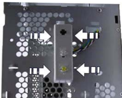
Fig. 15: Removing the switch/LED assembly
