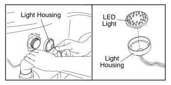
To replace the LED light, pull the old LED light out of the housing and insert a new LED light. Re-attach the light housing to the spa shell. Re-attach the access panel to the spa.
