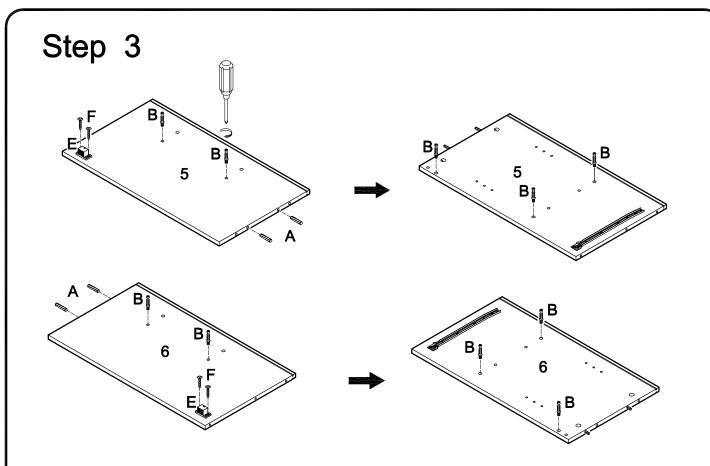
Screw cam bolts (B) and insert dowels (A) into panels (5,6). Attach door stoppers (E) to panels (5,6) using round-head screw (F). Flip panels (5,6) over and screw in cam bolts (B).
