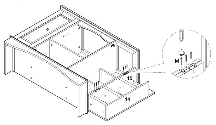
Attach the door (14,15) assembly to the stand assembly at hinges (L) using large screws (M).
