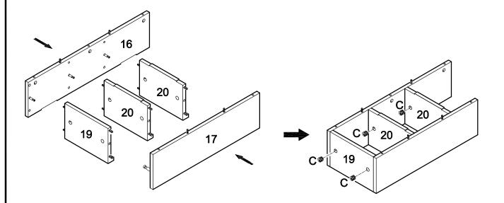
Attach shelves (19,20) to panels (16,17) using cam bolts and dowels as guides. Insert cam locks (C) into shelves (19,20) and tighten with a screwdriver. *Note that two cam locks will be inserted into each shelf.*
