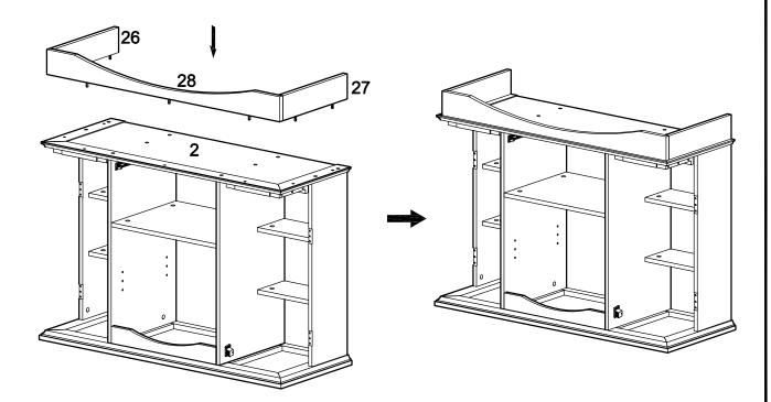
Attach the base assembly from Step 7 to the frame assembly by inserting the dowels of the base assembly into the pre-drilled holes of bottom panel (2).
