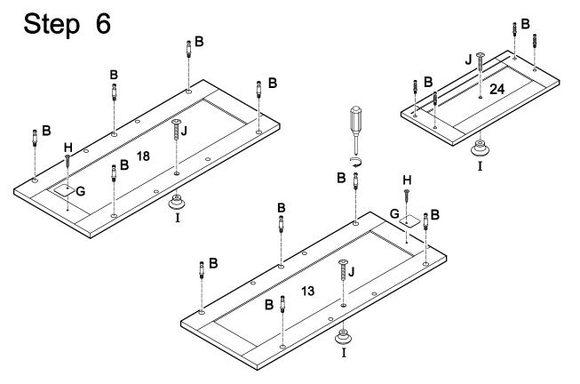
Screw cam bolts (B) into doors (13,18) and drawer front (24). Attach handles (I) to doors (13,18) and drawer front (24) using small bolts (J). Attach door stopper plates (G) to doors (13,18) using small screws (H).
