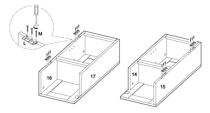
Attach hinges (L) to panels (15,16) using large screws (M).
