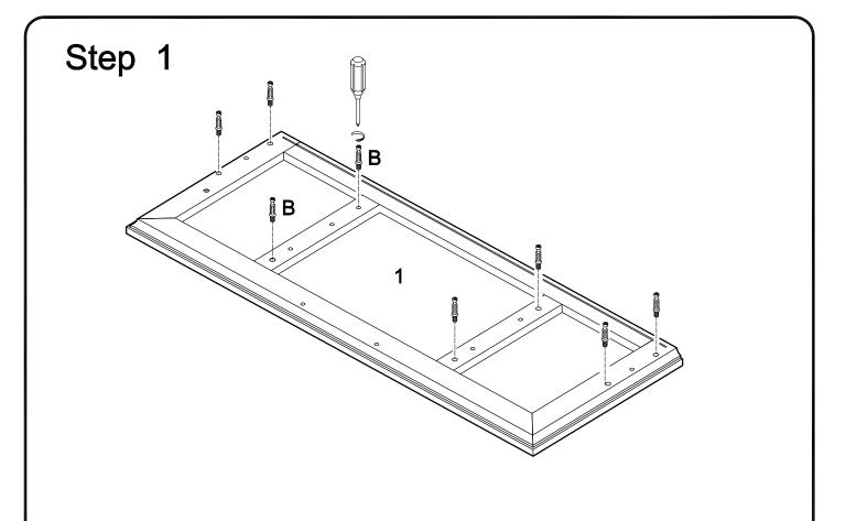
Screw cam bolts (B) into top panel (1).
