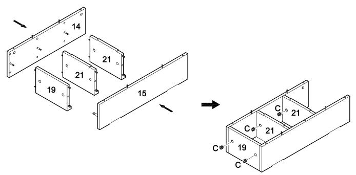
Attach shelves (19,21) to panels (14,15) using cam bolts and dowels as guides. Insert cam locks (C) into shelves (19,21) and tighten with a screwdriver. *Note that two cam locks will be inserted into each shelf.*
