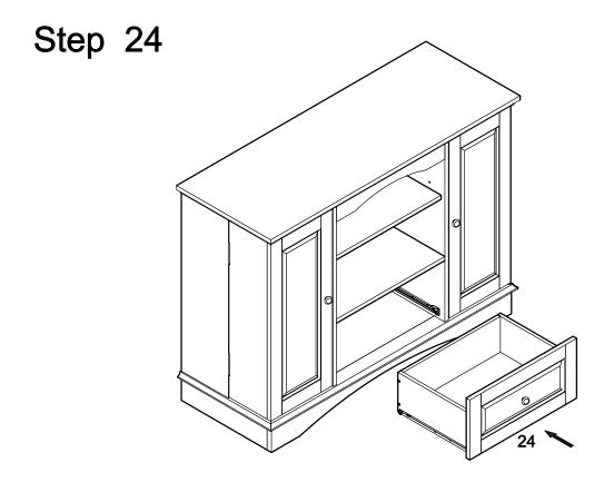
Carefully slide the drawer into the stand assembly.
