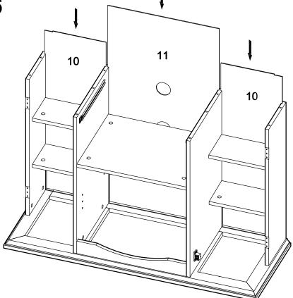
Slide back panels (10,11) into the frame assembly. Note that the back panels will slide down in the grooves along the back of the frame assembly.
