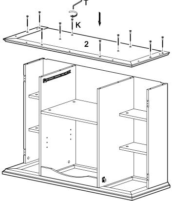
Attach bottom panel (2) to the frame assembly using large bolts (K) and wrench (T).
