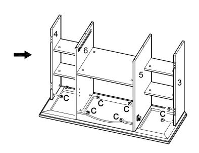
Attach the frame assembly from Step 14 to top panel (1) using cam bolts and dowels as guides. Insert cam locks (C) into panels (3,4,5,6) and tighten with a screwdriver.
