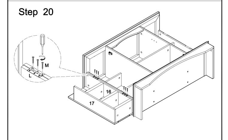
Attach the door (16,17) assembly to the stand assembly at hinges (L) using large screws (M).
