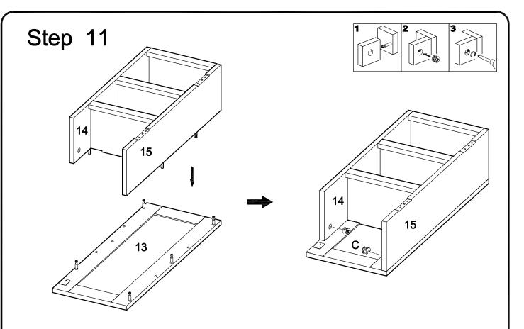
Attach the shelf assembly from Step 9 to door (13) using cam bolts and dowels as guides. Insert cam locks (C) into panels (14,15) and tighten with a screwdriver. Note that two cam locks will be inserted into panel (14) and three will be inserted into panel (15).
