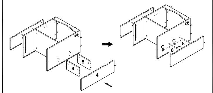
Attach shelves (8) to the opposite side of the frame assembly from Step 12, then attach panel (4) to shelves (8) using cam bolts and dowels as guides. Insert cam locks (C) into shelves (8) and tighten with a screwdriver. Note that two cam locks will be inserted into each shelf.
