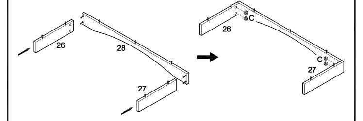
Attach slats (26,27) to slat (28) using cam bolts as guides. Insert cam locks (C) into slats (26,27) and tighten with a screwdriver.
