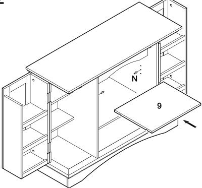
Insert shelf support pins (N) into the stand assembly at desired shelf height. Carefully place shelf (9) onto shelf support pins (N).
