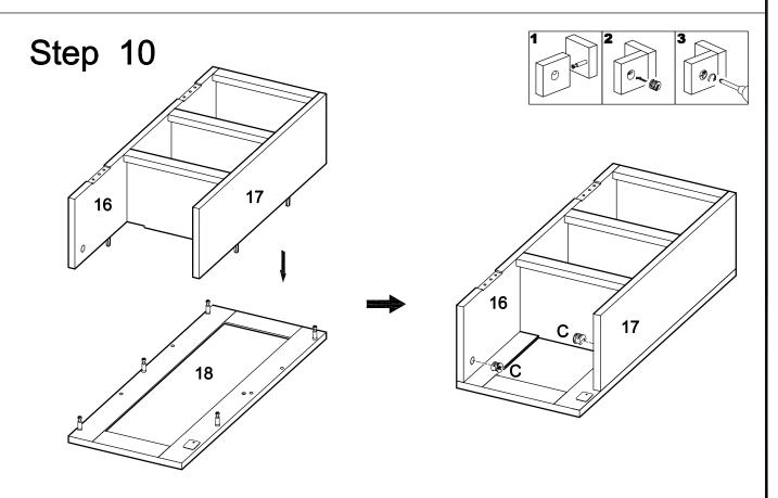
Attach the shelf assembly from Step 8 to door (18) using cam bolts and dowels as guides. Insert cam locks (C) into panels (16,17) and tighten with a screwdriver. Note that three cam locks will be inserted into panel (16) and two will be inserted into panel (17).
