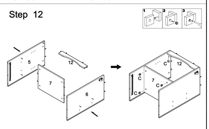
Attach panels (5,6) to panel (7) and slat (12) using cam bolts and dowels as guides. Insert cam locks (C) into panel (7) and slat (12) and tighten with a screwdriver. Note that four cam locks will be inserted into panel (7), and two will be inserted into slat (12).
