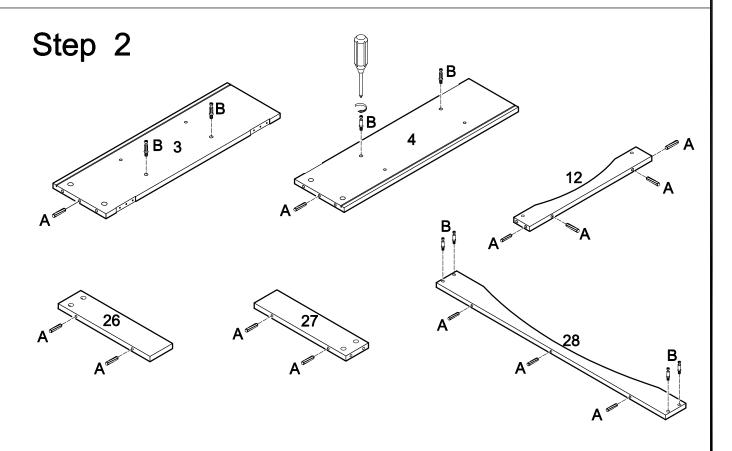
Screw cam bolts (B) into panels (3,4) and slat (28). Insert dowels (A) into panels (3,4) and slats (12, 26,27,28).
