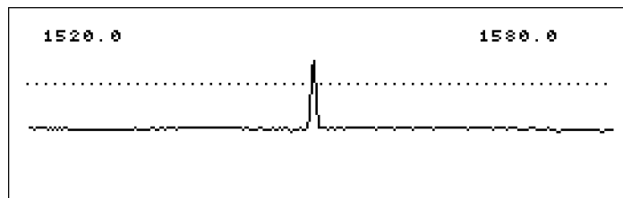
PRBS modulation graph showing raised noise floor.
