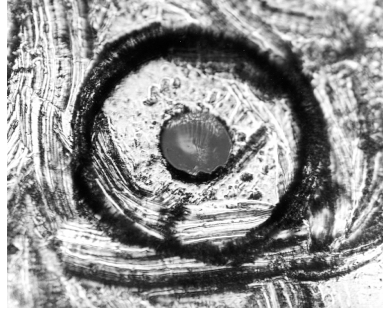
Figure 2-8. Damage from improper cleaning.
