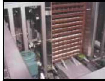
Oil Impregnated Nylon Basket Stack Transfer Roller System and Transfer Pusher for Durable and Smooth Stack Transfer
