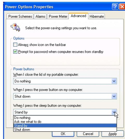
“Hibernate” is the same as Suspend-to-Disk (STD) and stores your current data and status on the hard disk drive. By doing this, RAM does not have to be periodically refreshed and power consumption is greatly reduced but not completely eliminated because certain wake-up components like LAN and modem needs to remain powered. “Hibernate” saves more power compared to “Stand by”. To operate: Enable hibernation in “Power Options” and select “Start” | “Shut down”, and “Hibernate”.
