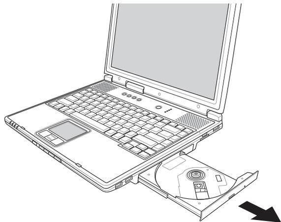
3. Hold the disc by the edge and face the disc's printed side up. Push down on both sides of the disc's center until the disc snaps onto the hub. **The hub should be higher than the disc when correctly mounted.**
