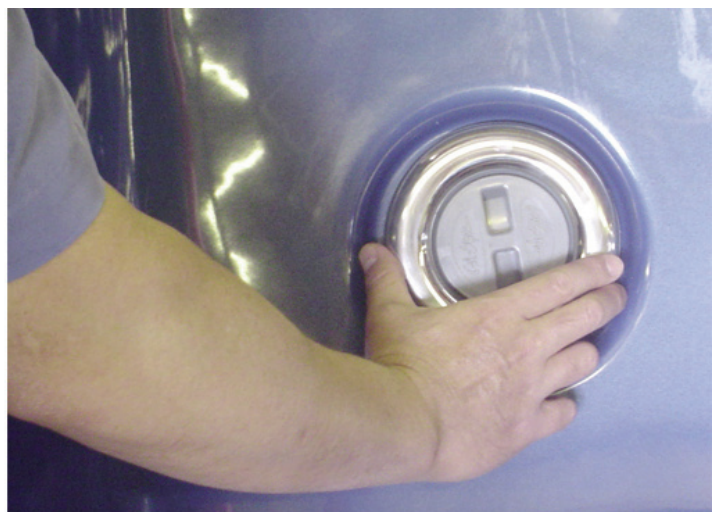
Figure 11. Rotating an adjustable jet
