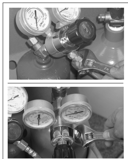
Figure 3 - Acetylene Connection (top) and Oxygen Connection (bottom)
