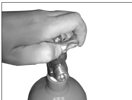
Figure 1 - Cracking the Cylinder Valve
