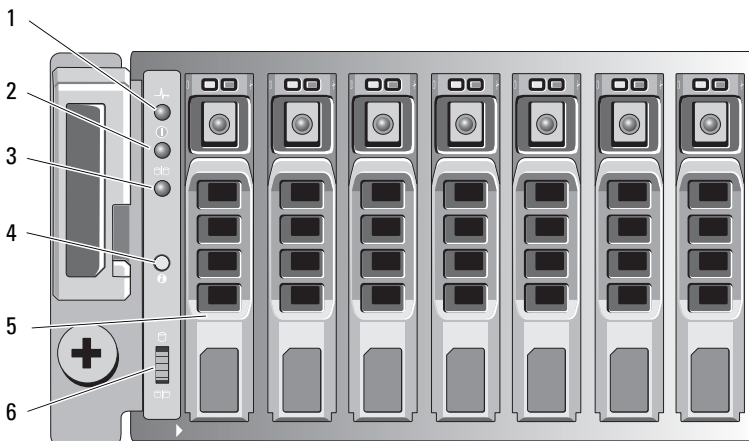
Figure 1-2. Front-Panel Features and Indicators—Dell PowerVault MD1220
