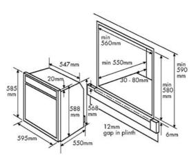
i) When installed in a typical 600mm deep built in housing unit, the false back should be removed from the housing unit to provide the necessary depth for installation.
