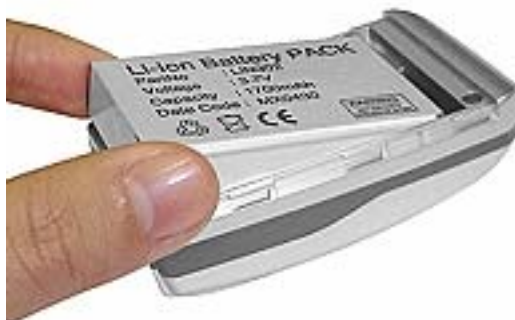
Replacement of Li-ion battery
