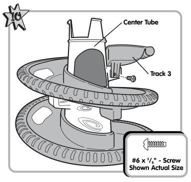
Insert a #6 x <sup>3</sup>/<sub>8</sub>" screw through the hole in track 3 and into the tube. Tighten the screw with a Phillips screwdriver.
