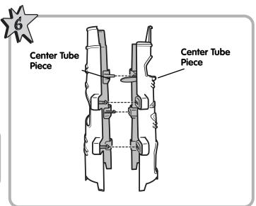
• Insert and "snap" the tabs on one of the center tube pieces into the slots in the other center tube piece.
