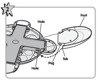
Insert the tabs on on each edge of a foot under the edge of the base so that you can fit the pegs on the foot into the holes on the bottom track.
