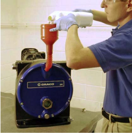
Figure 4 Fill Pump With Hose Lube
