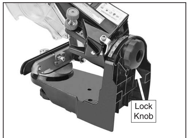
Figure 10. Swing arm lock knob installed.
